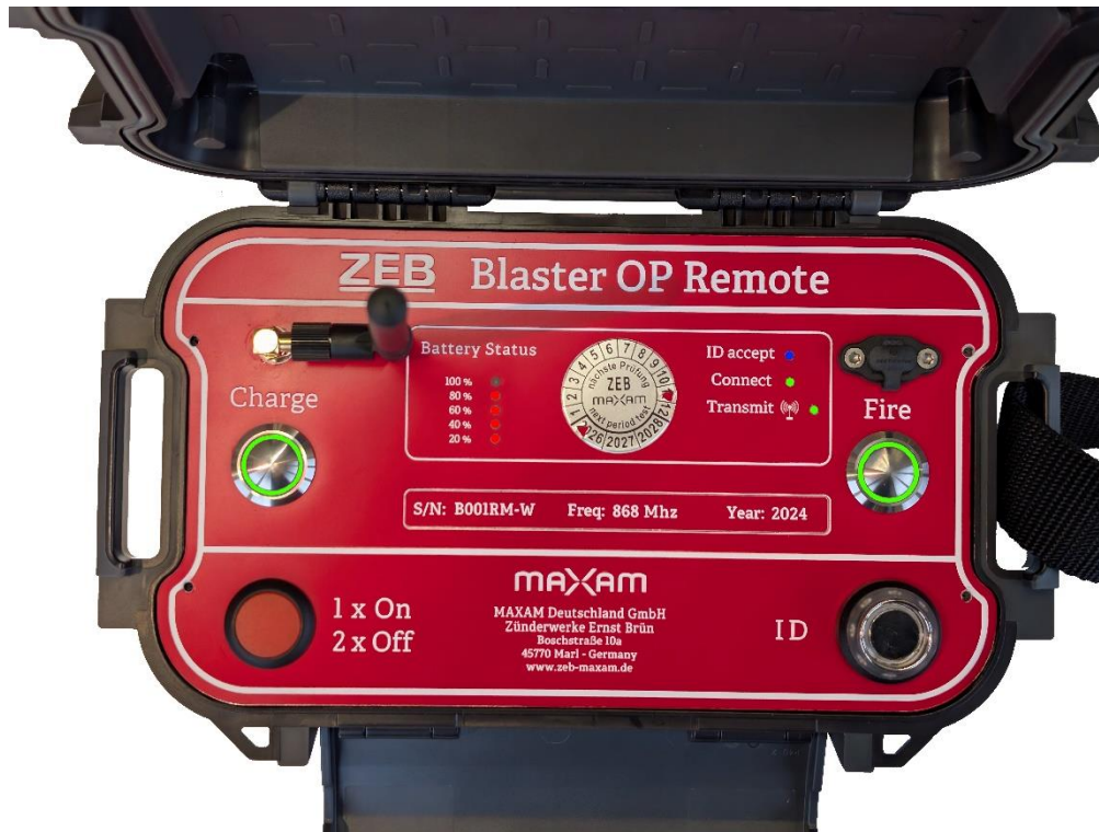
Remote shows a connected state and ready to fire – (ID-Chip missing) for light symbolization
